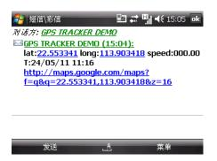
Tracking location, When no GPS signal, the SMS includes the last valid latitude & longitude as well as the LAC code of current position, the LAC code can be input in the column of "manual track" menu of web platform to check
